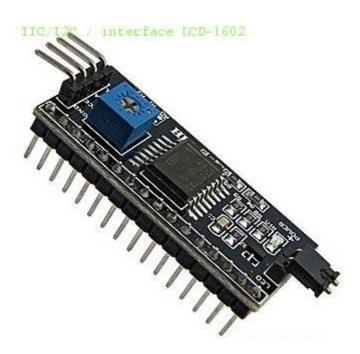
Arduino 1602 I2C interface four line 1602 screen
